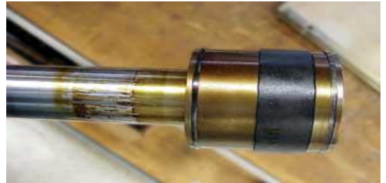
Illustration 2: Oxidized alteration sludge of oil is very difficult to remove
