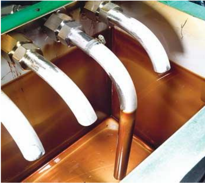
Illustration 1: Oxidative alterations adhering to the wall surface and inside the piping in large quantities
