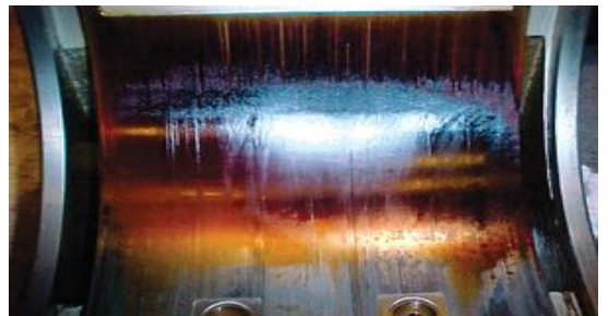
Illustration 3: With the spool of the valve that malfunctioned Oxidative alterations worn
