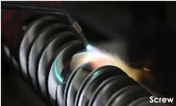
Manufacture Methods : PTA/HVOF/ARS SPRAY
